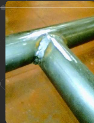
Welded Cod Mouth Joint
