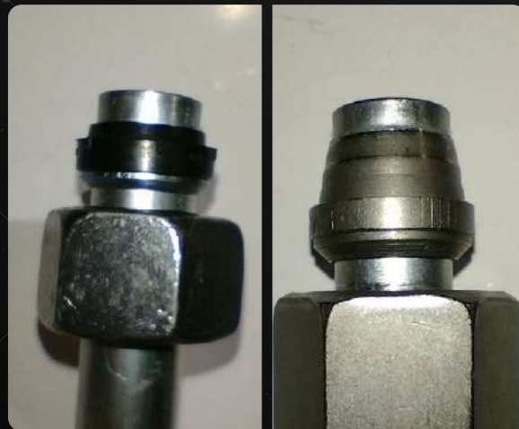
Installed fittings (Note EO2 on the left with soft seal)
