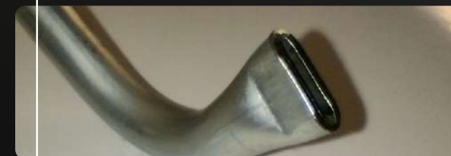
Flattened end (used as a spray nozzle)
