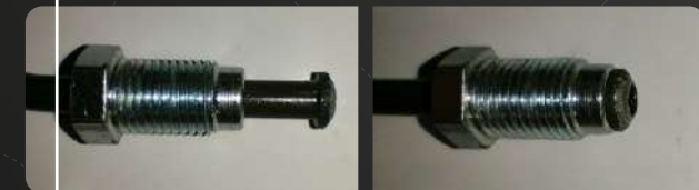
DIN Single Mushroom (Note 90-degree back face of flare)
